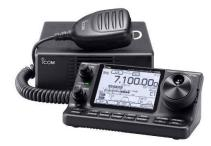
Many of our club members have purchased the ICOM-7100 Multi-Band & Multi-Mode transceiver which is an excellent choice. The IC-7100 capabilities include DSTAR digital voice which is commonly used on the VHF/UHF bands. DSTAR is also available on the new ICOM IC-9100 & IC-705 transceivers.
