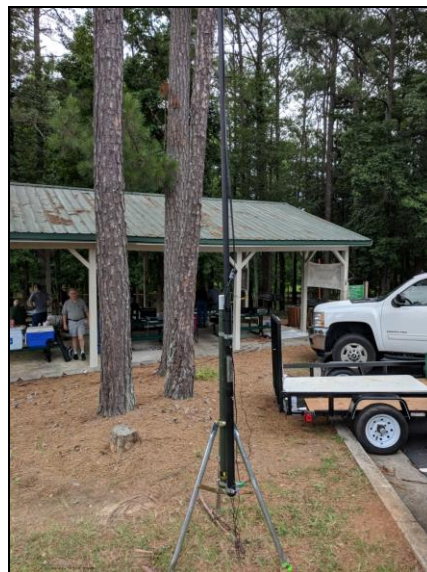
31' FG Vertical w/counterpoise & G5RV attached to the top
