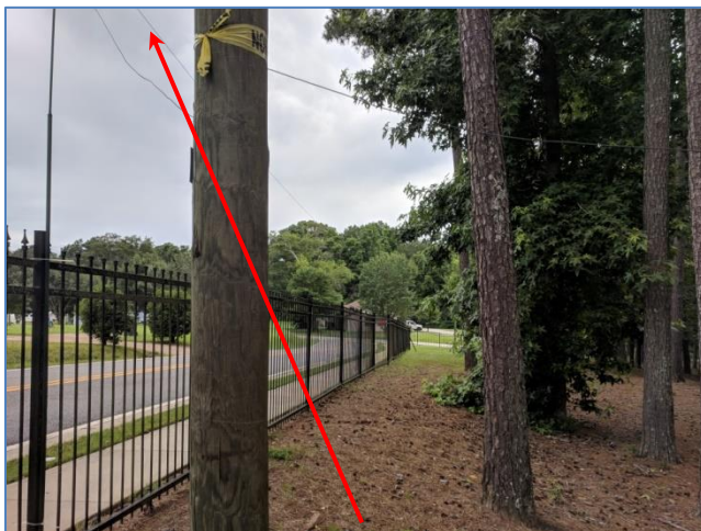
KM4IKO's 117ft EFLW antenna held up with garden sticks tie-wrapped to fence
