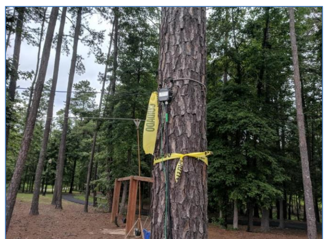
EFLW Balun bungied to a tree with tri-band rotatable dipole in background
