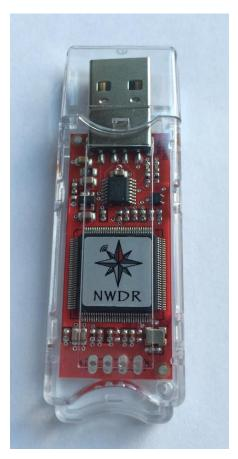
The NWDR ThumbDVTM adds D-STAR DV capability to your computer or laptop allowing you to get on the D-STAR network without a radio.
